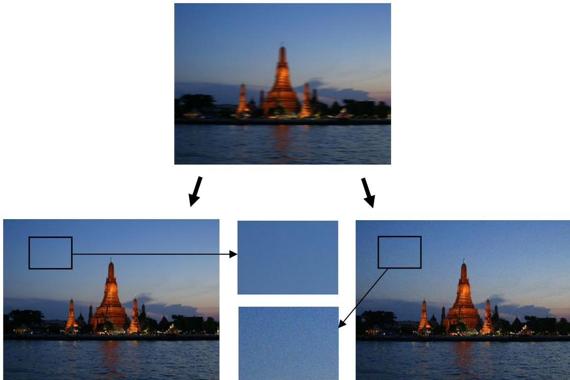
Fig. 1. Difference in image quality between image stabilizer and motion blur reduction
